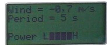
Do notice that at the bottom of the display screen, 4 little black blocks appear between L (=low) and H (=high), indicating that the voltage is still sufficiently high. Each time one of these blocks disappears; the voltage is decreasing until none of these blocks are left. This implies that the battery will have to be recharged.
