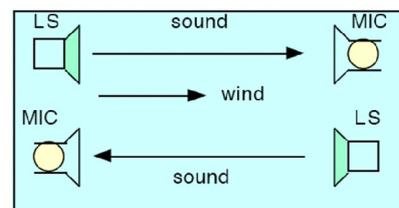
By measuring and registering the difference in speed between the sonic waves, which are travelling along with the wind, and the ones, which are travelling against it, we can very accurately determine the wind velocity.
